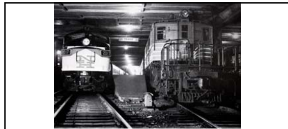
Above: at the foot of Tracks 20 and 21, the newest in locomotive technology ( New Haven Railroad's EMD FL9 on the left, built 1956-1960) and some of the oldest ( New York Central's T-3 class of electric on the right, built 1929-1930). The New Haven Railroad served GCT as well as the Pennsylvania Station . Both required the use of a third rail to enter the tunnels which led to EMD developing a "dual-mode" locomotive that could run off electric or diesel. A total of 60 FL9's were built for the New Haven, with more than half surviving to the Metro-North era. The last FL9 was retired in 2009, with many surviving at museums and tourist railroads throughout the eastern U.S. 474
